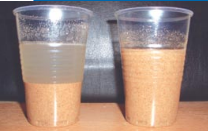
Clearbore solution treated with Calcium Hypochlorite bleach (left) compared to untreated (right)
